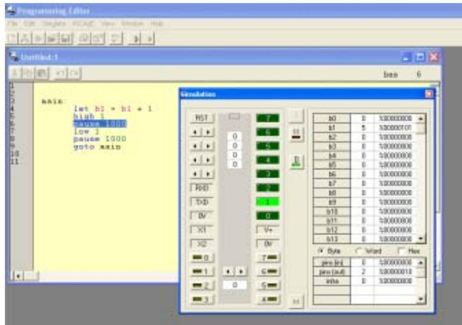
To simulate the program simply click the Simulate>Run menu. Each line of the BASIC code will be highlighted as it is processed, and an on-screen graphic shows the status of all input and output pins.
